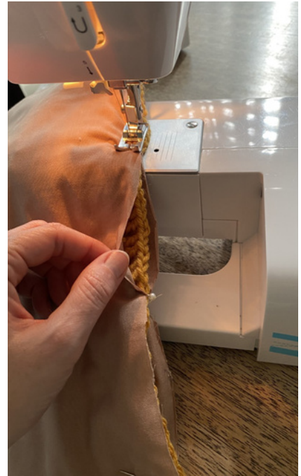
Be sure waffle panel is being stitched between fabric panels. May have to stretch gently to fit.
